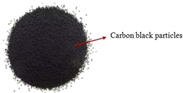
Figure 2. Carbon black wood apple shell particles. [Color figure can be viewed in the online issue, which is available at wileyonlinelibrary.com .]
